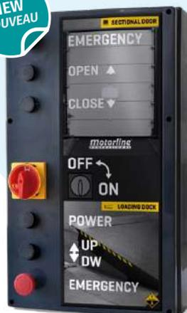
Electronic control board combined in a synchronized and safe way. Includes buttons to **open and close the gate**, button to **open/collect the dock leveler**, emergency and general cut-off buttons. This control board does not allow the dock leveler to be opened if the door is closed and, vice versa, it does not close the door if the leveler is open.
