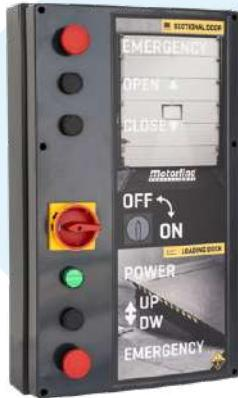
Electronic control board combined in a synchronized and safe way. Includes buttons to **open and close the gate**, button to **open/collect the dock leveler**, emergency and general cut-off buttons. This control board does not allow the dock leveler to be opened if the door is closed and, vice versa, it does not close the door if the dock leveler is open.
